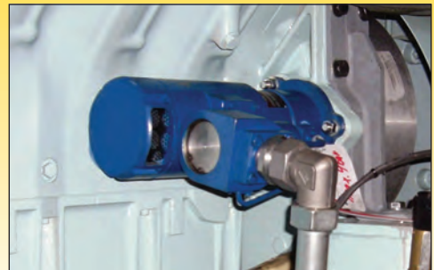
T25 installed on MAN D2842.
