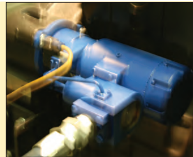
One hose, two wires, and 3 bolts and T25 is installed.
