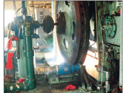
Model T100-B outboard-mounted starter on a slow-speed spark-ignited engine.
