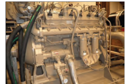
T106-F installed on Caterpillar 3412 engine.
