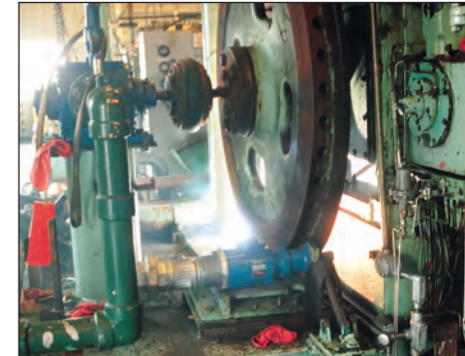
Model T100-B outboard-mounted starter on a slow-speed spark-ignited engine.
