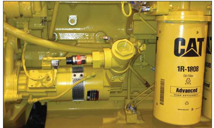
TurboStartTwo on Caterpillar C32 engine.
